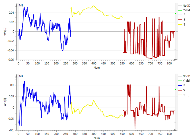
Figure 9: Loadings of the first component (top, R^2 of 0.497 and Q^2 of 0.364) and of the second component (bottom, R^2 of 0.341 and Q^2 of 0.165) given against batch maturity for each variable (pressure as blue, temperature as yellow, and agitator speed as red) for the filtration step in the FP process.
